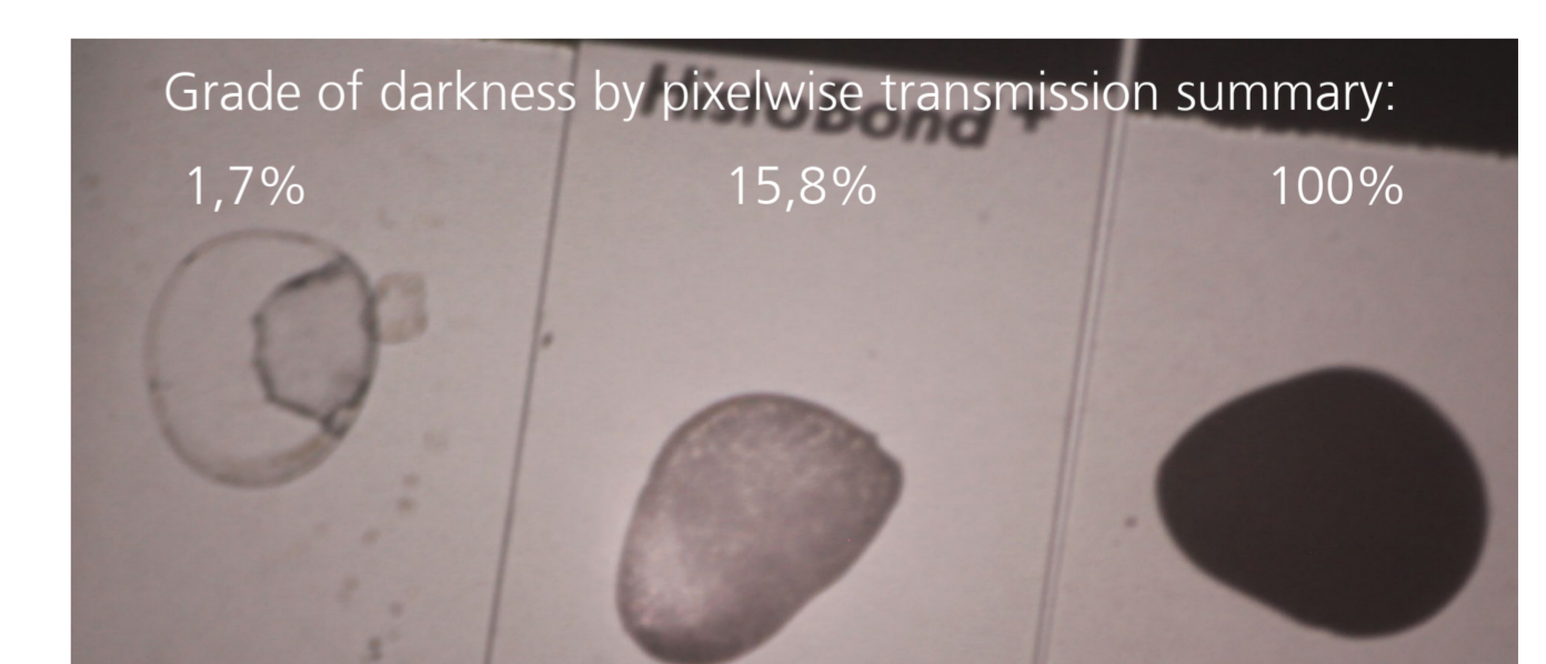
Absorption (lower right image) represents total dry mass of all non-volatile uremic toxins. It is fairly similar to small molecule reduction found in lab on that identical fluid samples using pixelwise integration and Lambert-Beer's law. This indicates heavy molecules to be removed either.
